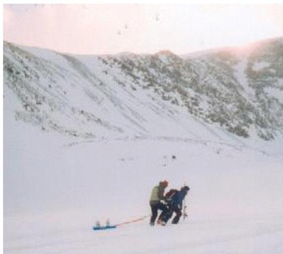
**Figure 6.** GPR polarization survey conducted on March 31<sup>st</sup> 2003 in the ablation area of Storglaciären. A commercial RAMAC GPR device (Malå Geoscience, Sweden) operating with two unshielded 200 MHz dipole antennas mounted on a plastic sled were used. A scientist was pulling the plastic sled while the radar operator was controlling the data collection with a laptop. Photograph courtesy of Fay Campbell.
