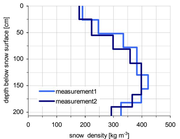
Fig. 4: Density profile at Pit 1 near stake 18 (30.03.2003)
